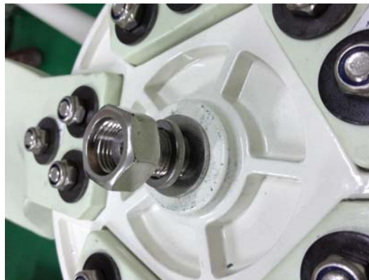
② Place the hub with blades onto the rotor shaft and “spin” it completely onto the turbine alternator shaft, then place in sequence of flat washer, spring washer and hex nut.
