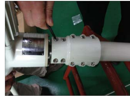
⑥ tighten the nut to 9N.m
