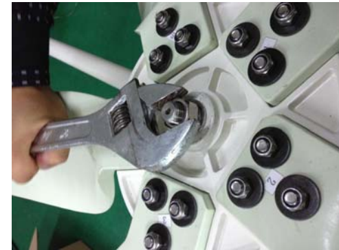
③ Fully tighten the nut to 154N.m
