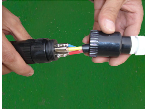
⑤ Screw up the cable cover.
