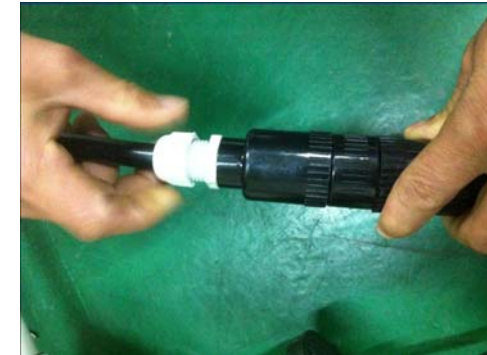
⑥ Screw up the waterproof cover.
