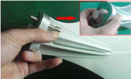
④ waterproof pad between tail and generator, use M8 bolts to fix the tail vane.
