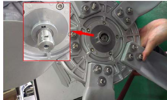
② Place the hub with blades onto the rotor shaft and “spin” it completely onto the turbine alternator shaft, then place in sequence of flat washer, spring washer and hex nut.
