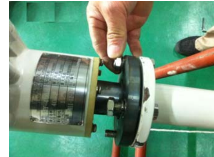
③ Place flat washer, spring washer and nut, tighten the nut to 60N.m
