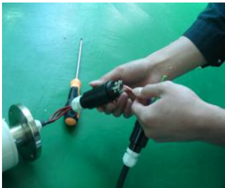
④ Connect the three-phase lead wires into the terminals (make sure three phases are not short circuited)
