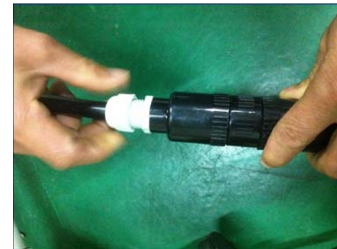
⑥ Screw up the waterproof cover.
