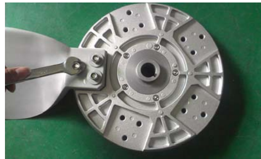
⑤ Place blade, flat washer and locknut, and tighten the nut to 18N.m
