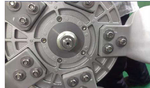
③ Fully tighten the nut to 290N.m
